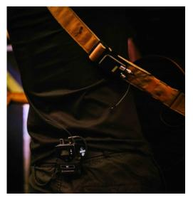
The SK 6212 mini-transmitter is attached to the guitar strap
